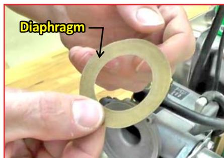
Inspect the Diaphragm for any cracks, folds or tears. Replace Diaphragm if damaged.
