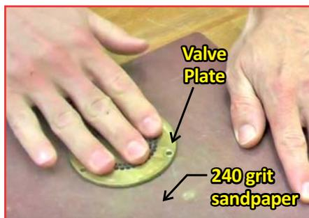
Clean and recondition the Valve Plate surfaces with a 240 grit sandpaper on a flat surface.
