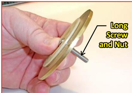
Keep Diaphragm centered over the Valve Plate holes. Reinstall the assembly screw and nut.
