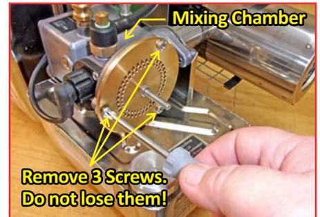
Remove the 3 mounting screws that hold the Air Intake Valve assembly to the Mixing Chamber.
