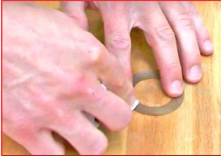
Use a soft clean cloth and a flat surface to carefully clean both sides of the Diaphragm.
